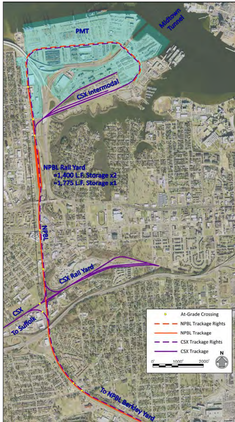
Figure 4 – PMT Overall Rail System
