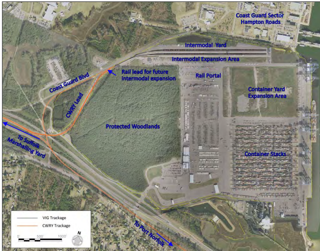
Figure 22 – VIG On-Dock Rail System
