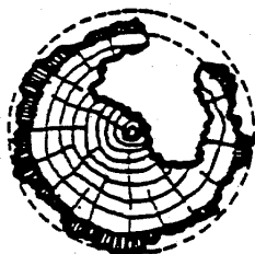
55-85 % REMAINING MAXIMUM DAMAGE
