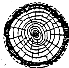
90-95 % REMAINING MINIMUM DAMAGE
